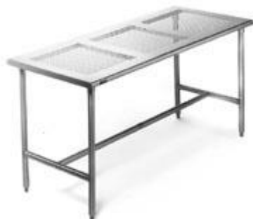
14 Gauge 304 Grade Cleanroom Stainless Steel Tables Perforated top; allow a minimum 40% laminar flow
